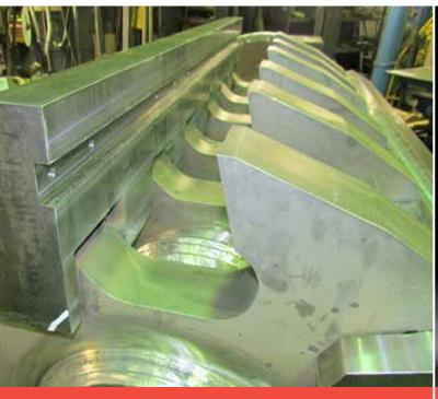
Detail of Prise™ 3 rotor with hammers
