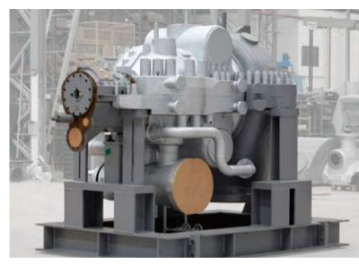
SST-300: 26 MW back pressure turbine for a sugar and ethanol plant in Brazil
